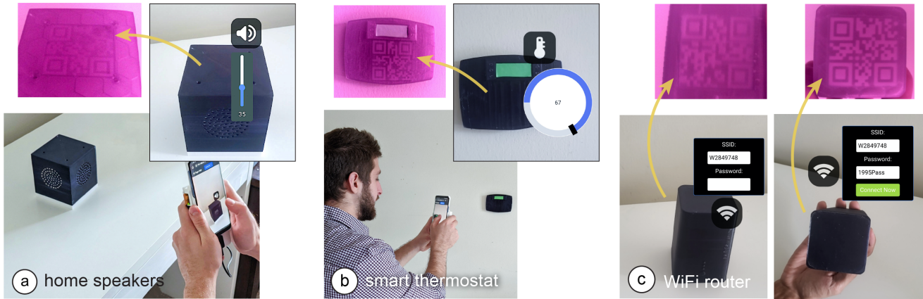
Figure 7: Controlling appliances using a mobile AR application. The user points at (a) the home speakers to adjust its volume, and the (b) thermostat to adjust the temperature. The infrared camera in the phone’s case identifies the appliances by reading the embedded QR codes. (c) Pairing a phone with a WiFi router, whose SSID is visible from all sides but the password is visible only from its bottom.
